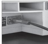
Connect to 130kHz, 95–265Vac. Make sure the power cord is very firmly pushed into the MAINstage's receptacle.
